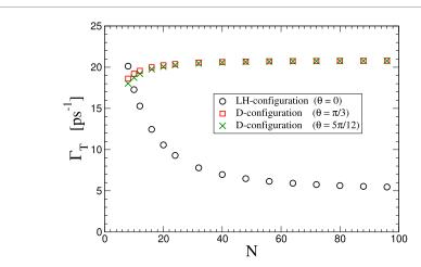
**Figure F1.** Dephasing rate (see equation (F.6)) vs the system size N for LH-configuration ( $\theta=0$ ) and D-configuration ( $\theta=\pi/3, 5\pi/12$ ). Parameters:  $E_R=200~{\rm cm}^{-1}, \omega_c=333~{\rm cm}^{-1}, T=300~{\rm K}$ .
